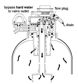
Timer/switch action again allows the motor to turn the rotor & disc to place the valve in BACKWASH, stopping water flow to the nozzle. Water is routed down and out the bottom distributor, up through the bed, and out the top distributor to the drain. The fast flow (controlled by a flow plug in the drain fitting) flushes dirt, sediments, iron deposits, remaining brine and hardness to the drain.
